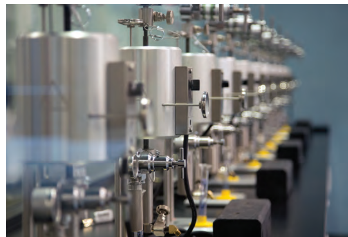
A row of HPHT fluid loss test cells in the Newpark Technology Center laboratory.
