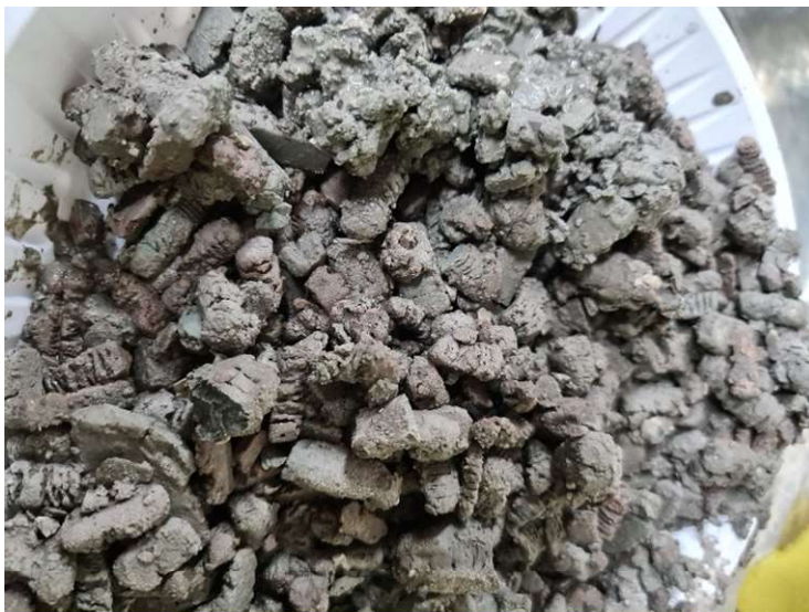
Figure 1: Cuttings from the well illustrating superior inhibition achieved from careful design of the customized HPWBM
