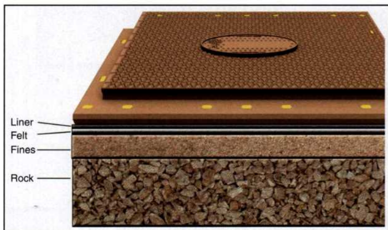
Traditional Multilayer Liner Protection System
