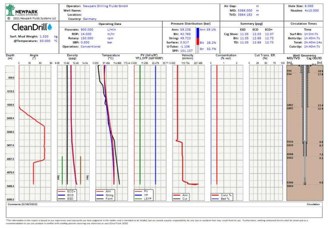
As a result of Newpark's comprehensive tests, the decision was taken to change the drilling fluid to a salt-saturated fluid weighted with barite, formulated with 2% of Newpark's proprietary Avagreenlube™ ester-based lubricant.
