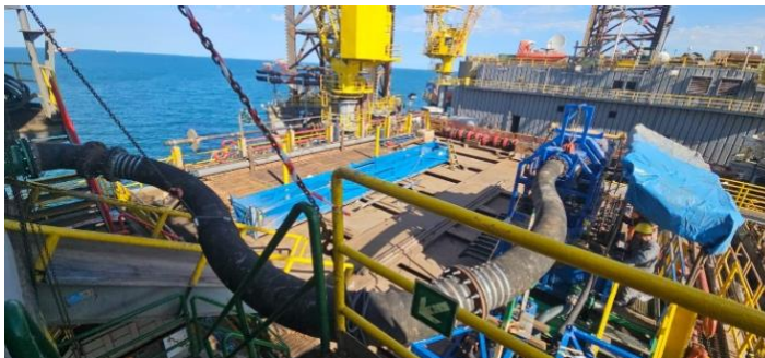
Figure 2 - Swarf unit package & flexible feeding pipe
